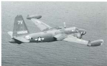
(Below) P2V-6 Neptune from NAS Glenview, Illinois in overall Semi-gloss Seaplane Gray. Reserve band of International Orange is partially visible just forward of the horizontal stabilizer. The "7V" tail code indicates NAS Glenview. (Eric Lundahl via Harry Gann)
