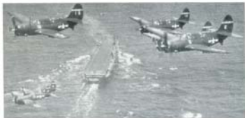
(ABOVE) SB2C-5s and F4U-4s of Air Group 75 with horizontal bands on their vertical tail surfaces. Color of bands appears to be Insignia Red on the Helldivers and either Insignia White or Light Yellow on the Corsairs. Carrier is USS FRANKLIN D ROOSEVELT (CVB-42) in mid-1946. (USN)
