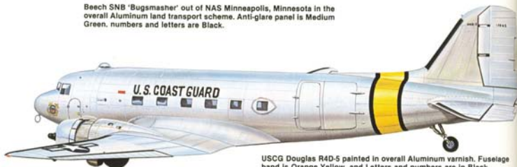
USCG Douglas R4D-5 painted in overall Aluminum varnish. Fuselage band is Orange Yellow, and Letters and numbers are in Black.
