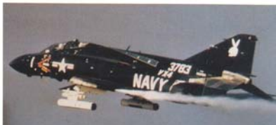
The experimental all Black F-4J Phantom II of VX-4, known as 'Vandy One', tested the anti-corrosiveness of the paint. 1973. (Jerry Kishpaugh)
