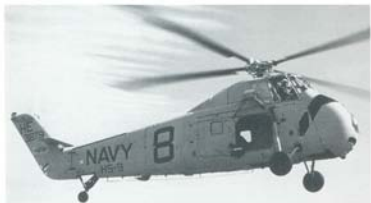
HSS-1 helicopter of Anti-submarine Squadron 9 painted overall Light Gull Gray, February 1958. Side and bow number (Black 8) was to be as large as possible without exceeding 48 inches except when two digit numbers were used. This was according to the directive issued on 9 March 1955, covering individual ASW helicopter ID markings. (USN via Harry Gann)
