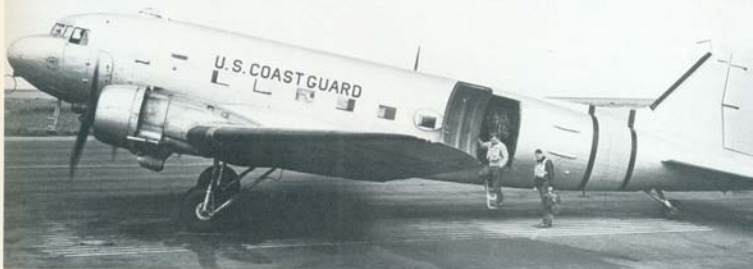
Douglas R4D-5 during early 1950. Eight of these were acquired by the Coast Guard between May of 1943 and July of 1944. Aircraft is overall Aluminum varnish with an Orange Yellow fuselage band outlined in Black. The branch of service marking is carried above the windows as ordered in SR-2G Amendment One. (USCG)
