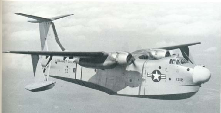
(Below) USCG P5M-2G Marlin 'T tail' from the Coast Guard Air Station, Elizabeth City, North Carolina in October 1956. The anti-glare panel is Medium Green. (USCG)
