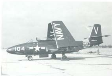
(Above) NAS Glenview, Illinois F2H-1 Banshee carries the oversized NAVY applied to the underside port wing. Maximum size was to be 30 inches. (Eric Lundahl via Harry Gann)
