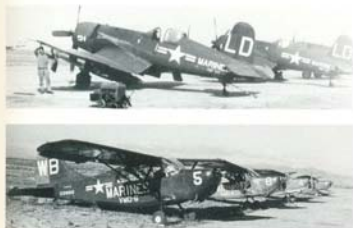
(Above) VMO-6 observation planes on Tonpo Airfield near Hungnam, Korea on 6 November 1950. Nearest plane is a Consolidated-Vultee TN-OY-2 and is painted overall Glossy Sea Blue. The other planes are believed to be OY-2s and are painted in the USMC land camouflage scheme, Olive Drab top surfaces over Light Gull Gray undersides. The "TN" designation was applied to training aircraft. (USMC via Rowland P. Gill)
