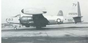
This Glenview P2V-6 carries the Fluorescent (High Visibility) Color Configuration scheme called out in MIL-C-18263(Aer) of 12 February 1959. Semi-gloss Fluorescent Red Orange was added to empennage, wing tips and forward section of aircraft for Hi-Viz. Balance of this Neptune's scheme is Insignia White fuselage top surfaces and Semi-gloss Seaplane Gray lower surfaces. (Eric Lundahl via Harry Gann)
