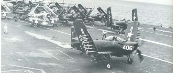
(Above) "Green Pawns" AD-6 Skyraiders on flight deck of FORRESTAL (CVA-59) in early 1956 during its Caribbean Shakedown Cruise. Tip of the vertical fins and rudders of VA-42 AD-6s are Glossy International Orange. That this is a period of change-over between the old and new scheme is obvious. Eight squadrons comprised Air Task Group 181 onboard CVA-59 at this time. (Douglas via Harry Gann)
