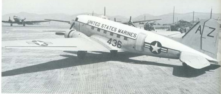
Douglas R4D-5 with newly applied solar heat reflecting Insignia White fuselage top as directed by SR-202 of 1 August 1953. Letters "AZ" are for HEDRON One, Korea. (USMC via Rowland P Gill)
