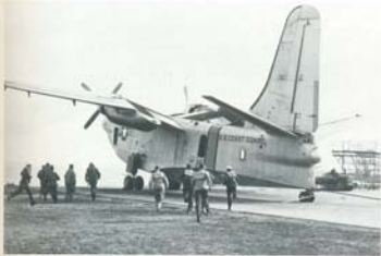
(Above) Crewmen scramble for their Martin P5M-1G Marlin seaplane called out on a search and rescue mission at USCG station at Elizabeth City, North Carolina in January of 1954. Orange Yellow stripe around fuselage with overall Aluminum varnish paint scheme. (USCG)
