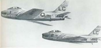
(Above) VF-122 FJ-2 Furies in flight on 6 December 1954 in the experimental natural metal scheme that was used from April 1952 until February of 1955. A few aircraft from each squadron tested the unpainted finish which was top coated with clear lacquer. Fuselage stripes, nose intake cowl and tail markings were Light Green and White. (USMC via Rowland P Gill)
