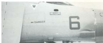
Close-up of air intake showing small 'danger' warning sign. (B R Jackson)
