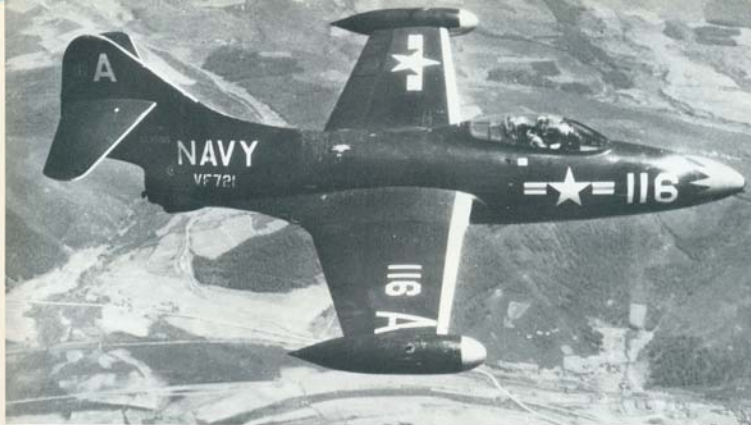
F9F-2B Panther of VF-721 from NAS Glenview, Illinois Reserve unit in flight over Korea in 1951. Squadron was activated for Korea on 20 July 1950 and went aboard USS BOXER (CV-21) in March of 1951. Nose trim is Insignia Red for first squadron. Leading edges of wing are natural metal. (USN via B R Jackson)
