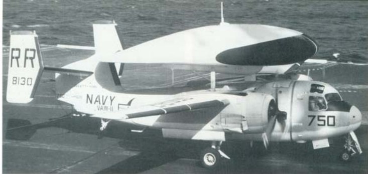
(Below) Grumman E-1B Tracer (WF-2) of VAW-11, WHISKEY detachment, being trapped aboard KITTY HAWK (CVA-63) on 22 October 1962. The E-1B Tracer was designated WF-2 Tracer prior to September 1962. At the time of this photograph the fuselage designator, WF-2, had not yet been changed. Color scheme is the standard Light Gull Gray over Glossy Insignia White. (USN via Harry Gann)
