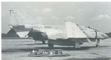
F-4S Phantom II (155767) of VF-171 from NAS Oceana, 2 October 1982. Very small "AD" tail code can be seen at top of vertical fin. Top-side colors are FS 35237 and 36320 over underside color FS 36375. This scheme was approved on 3 February 1982. (Douglas R Tachauer)
